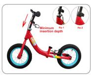
Step 3: Insert handlebar into fork tube, and tighten the screw with hex key as Pic 1, then put down the T bar cap as Pic 2, please note align handlebar and wheels
