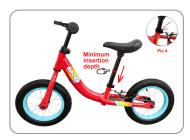
Step 4: Insert seat, then tighten the screw of clamp under the seat
