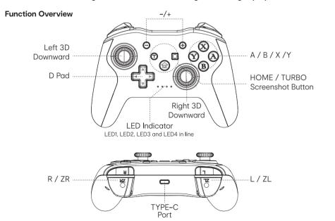
Press HOME button to wake-up controller. Press and hold HOME button to turn off controller
