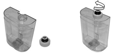
• Rotate the water tank so that the cap is at the bottom and then slide it down into the base unit as shown and push down until the latch locks it in place.
