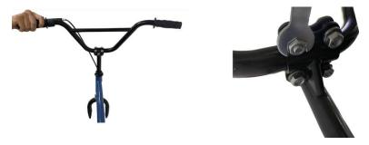
Move upward the handlebar, adjust to your desired angle, then tighten the four bolts and nuts using the appropriate wrench.
