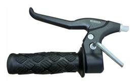
Using the allen key to loosen the lower screw on the brake lever, adjust the lever to your desired angle and then tighten the screw.
