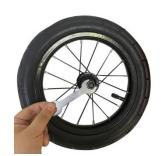
Remove the protection covers on the wheel. Loosen and take off the washers and nuts on wheel, then put the wheel into the fork. Install the washer and nut to fix one side of the wheel, tighten the nut using the appropriate wrench. Do the same installation on the other side. Please make sure the washer hook insert into the hole on the fork.
