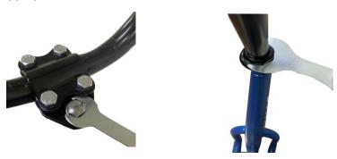
Tighten the upper stem pillar bolt using the appropriate wrench. Then tighten the head cup top using the appropriate wrench.
