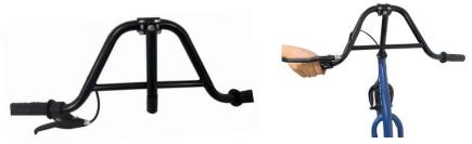
Remove the protection covers on the bracket. Make sure the brake lever is located at the left hand. Insert the stem pillar into the fork tube to the minimum insertion line, which is indicated on the stem pillar. Face the handlebar stem forward directly in line with the front wheel. Make sure the bracket is centred.
