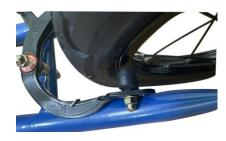
Regularly check the brake rubber is touching the rim to stop, not the tyre. Once find the rubber in displacement, loosen the screw using the appropriate wrench to adjust the rubber, make sure the rubber touch the rim to stop. Check the two sides rubber all the time.
