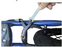
Using the appropriate wrench to loosen or tighten the screw on the rear brake. It controls the tightness of the brake cable. Adjust to your desired tightness but make sure the brake function will not be effected.
