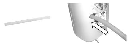
• Place the other end of the tube into a container or directly into a drain.
