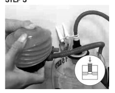
Press the spring valve again to close the valve, and connect the special nozzle equipped on the pump, then press the pump with hands or feet to inflate
