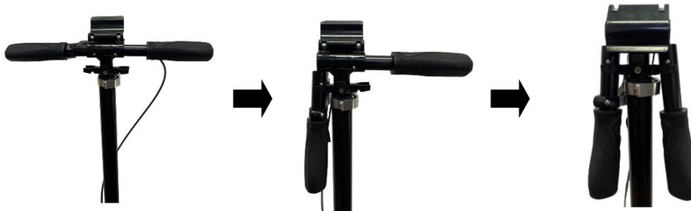
Step 3 Press and hold the lever of folding mechanism to loosen the transportation lock. Fold up the scooter by moving the handlebar stem towards the rear wheel until you hear transport lock click into place.
