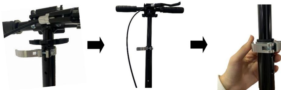
Step 2 Open the quick release. Use your thumbs to press both locking buttons in the handlebar grips and pull the handlebar grips outwards until they are completely released. Hang the handlebar grips into bracket properly. Then tighten the quick release.
