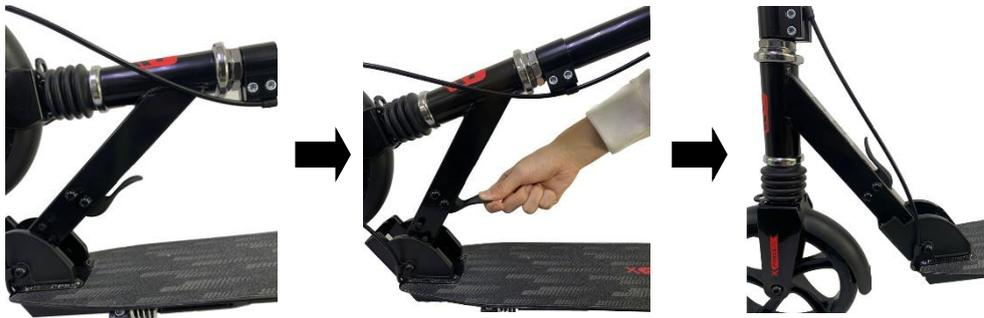
Step 2 Open the quick release. Insert the handlebar grip into the handlebar spring button of the handlebar stem. Use thumbs to press down both buttons until the grips can be easily pushed in. Turn the handlebar grips until the locking buttons are positioned in the two openings and hear them click into place. Then tighten the quick release.
