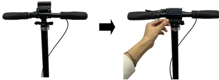
Step 3 Loosen the quick release by pushing the lever of the quick release lock until the lever is parallel to the handlebar grip. The handlebars can be locked into place at 2 different heights. Please adjust the height to your required height. Then tighten the quick release.
