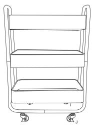
3. Assemble the bottom tray first, using (e)(f)(g) to connect the tray and tube frame together. Use the spanner (h) to fix the nut (g).
