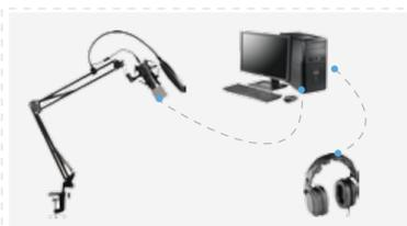
(8) Step 8, Connect the microphone with your computer, prepare a wired headphones to hear the voices from the microphone
