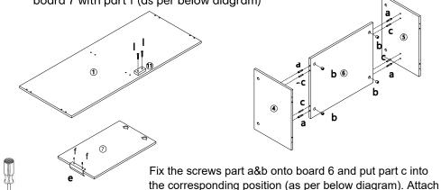
board 4 and 5 to board 6, and then fix the round screws
