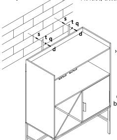
At last, attach the wall fixings onto the wall with part s&q&d
