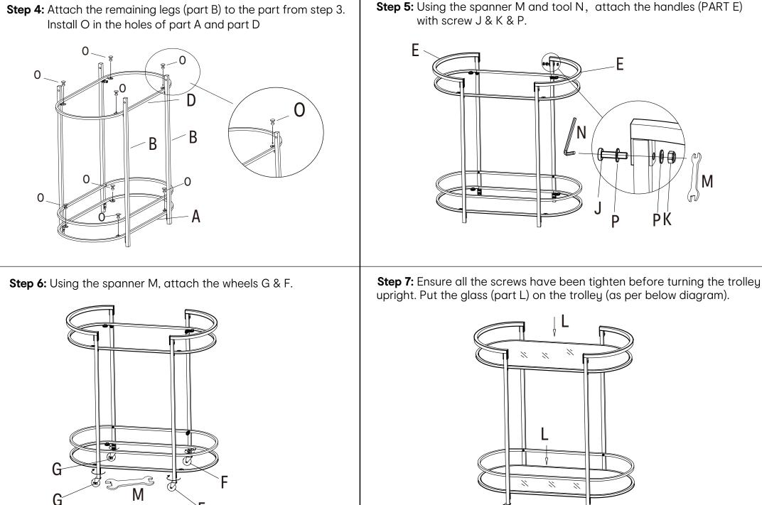
**Step 4:** Attach the remaining legs (part B) to the part from step 3.
