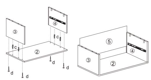
**Step 4:** Put part b & c into the corresponding position (as per below diagram) and fix screws a onto board ①. Join board ① to the part from. step 3 and fix part b with a screwdriver. Ensure all parts align.
