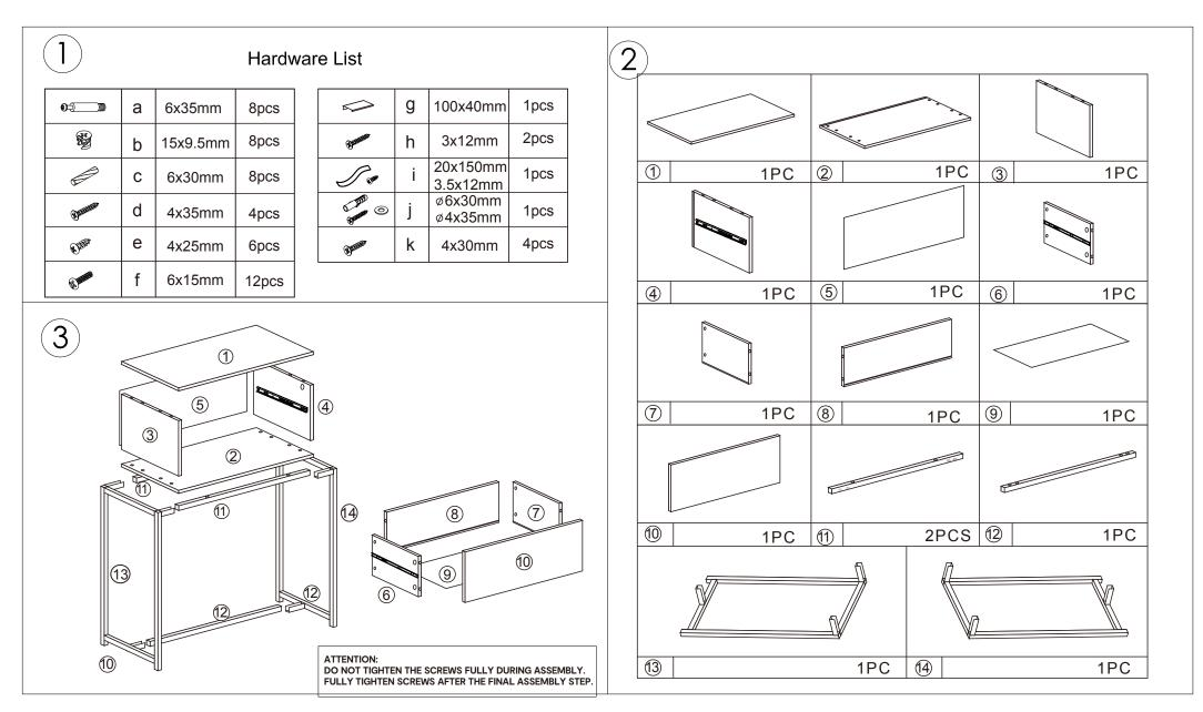
**Step 1:** Assemble board (6), (7), (8) with screws (Part k). Slide board (9) into corresponding position (as per below diagram). Ensure it is fully fitted in the groove.
