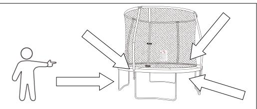
**Inspect prior to use** – check that the legs are properly attached and stable on the ground; no loose springs; mat and enclosure net are in proper place and in good condition with no tears.
