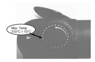
NOTE: When turning the temperature control knob clockwise, each dot point will increase the temperature by approximately 10°C up to a maximum temperature of 210°C.
