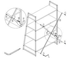
Step 5: Fasten the metal wire (Part B) and Board (Part D) with screws (part J).
