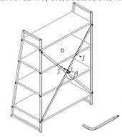
Step 6: Put screw (Part N) into the small hole of nylon tie (Part P) and across plastic anchor (Part O) to fasten to the wall. Fasten all screws firmly, assembly is now complete.
