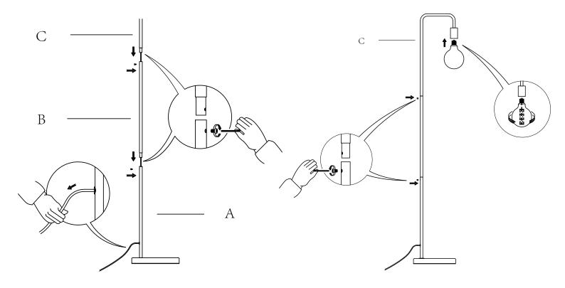
2. Insert the middle tube (B) to insert the bottom tube (A). Then take the bent tube (C) to insert the middle tube (B). Pull the cable gently through the bottom tube outlet.
