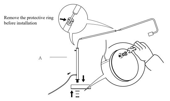
1. Insert the bottom tube (A) into the marble base. Put the rough surface of the flat washer, spring washer and the hexagon bolt in order to insert the bottom tube. Use the spanner to screw down the hexagon bolt. Ensure the cable exits from the back of the lamp.
